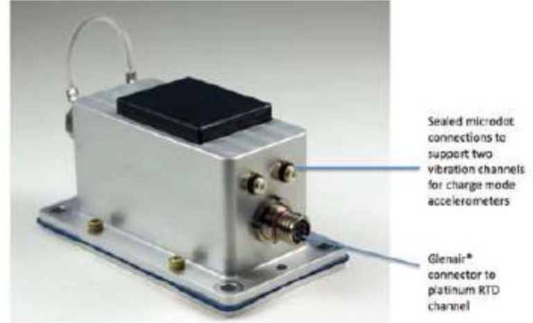
Figure 2. Energy-harvesting wireless sensor node for vibration and temperature monitoring.
